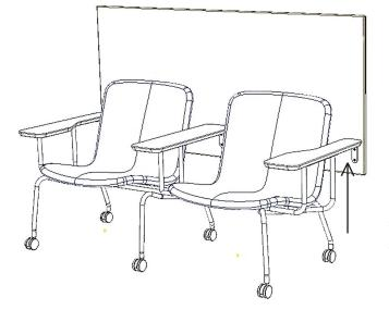
Start to assemble the back screen. Use the M6x20 mm screws into the T-nuts underneath the armrest tops.
