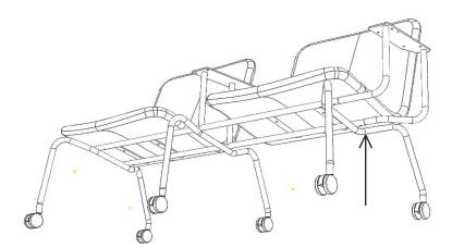
Secure them by screwing the M6x20 mm screws through the tubes into the armrest(s), 4 screws/armrest.
