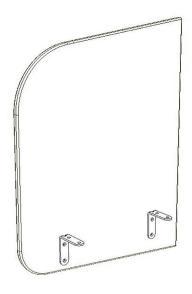
Fasten the brackets onto the screens with the countersunk M6x20 mm screws. Two brackets for the side screens and two or three for the back screen.
