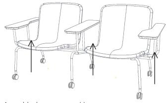
Assemble the armrest top(s) by screwing the M6x20 mm screws in the T-nuts from underneath. NOTE! If you are adding screens, don't tighten the screws until the screens are added.
