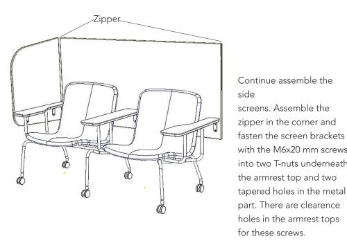
Finish the assembling by tightening the screws for the armrest tops.
