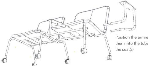
Position the armrest(s) by sliding them into the tubes underneath
